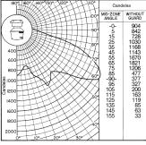
NOTE: Photometric data was developed using a 100 watt clear high pressure sodium lamp (9500 lumens). For other clear lamps, use the following conversion factors (multipliers):
